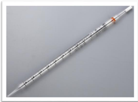
Pipette (glass/plastic) Transfer of measured volumes of solutions
